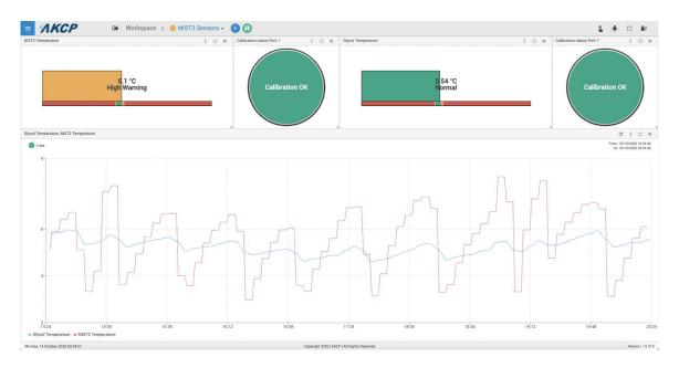
The NIST2 sensors feature 2x NIST traceable, calibrated temperature sensors and an internal calibration integrity check.
