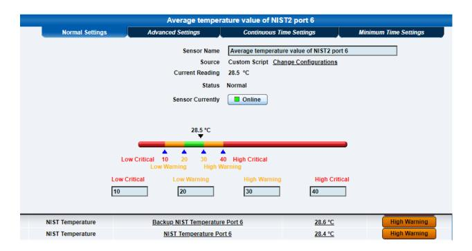
This is an example of the configured value averaging virtual sensor for the NIST2 sensor that is plugged on sensor port 6.
