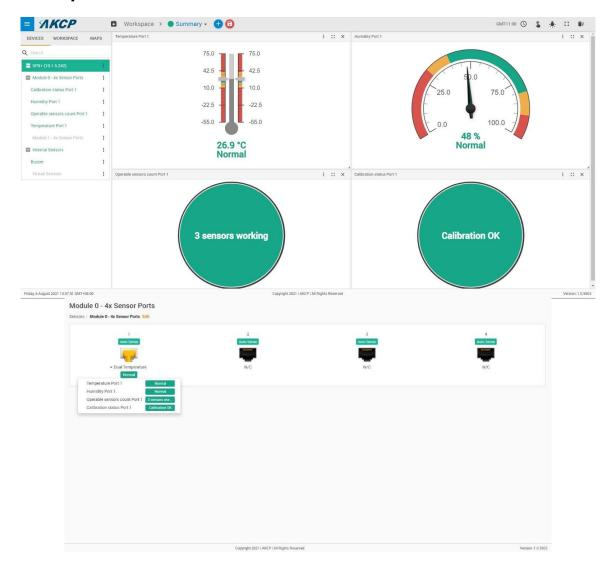
After plugging the NIST sensor to the main sensor port or Sensor4 module, the following sensors will be shown on the unit.
