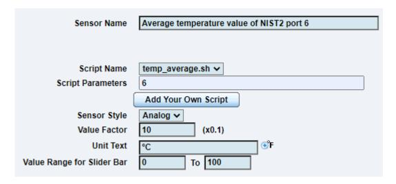
7. Configure sensor thresholds as desired.
